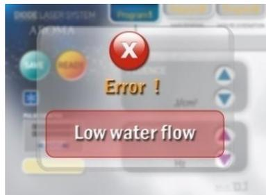
It happens when the cooling water is not circulated well.
