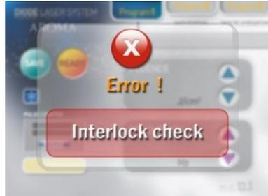
Interlock check error. Make sure that interlock switch is fastened in the back below
