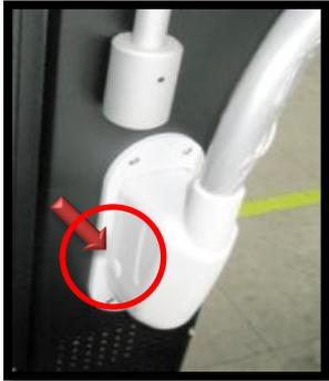
Connect handpiece connector by pushing both round buttons of it. After connecting, make sure it is connected well by pulling it slightly.
